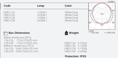
FMD Fixtures are composed of batten (FMS) and reflector
