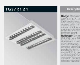
Body: Manufactured with 6114, A1 quality DKP steel sheet and coated with min. 80 micron thick epoxy polyester electrostatic powder paint. powder paint.
