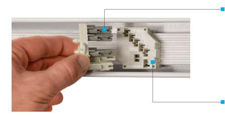
The phase selector is a special type socket. When selecting the phase, the 5-wire system is neutral and the earth contacts are fixed to the energy receiving apparatus. One of the three phases can be selected by moving contact.
