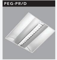
Body: 0,6 mm thick, 6114,A1 quality DKP steel sheet is used in manufacturing. The body is coated with min. 80 micron thick epoxy polyester electrostatic powder paint. (Standard color RAL 9016) **Reflector:** The reflectors
